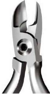
B-12-5713 T/C 12.5 cm/ 5" Hard Wire Cutter, Flat Back Cutting capacity up to .020 round, Arch wire up to .022 x .028 and all sizes of ligature wire and pins.
