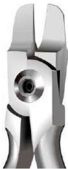
Tweed B-12-4611 T/C 11.5 cm / 4½" Rectangular Arch Pliers, Tweed Style Forming plier for square or rectangular wires. The blades are designed to be parallel at .020" ( 0.51 mm ) opening. The working edges are carefully diamond-honed to prevent wire scoring.
