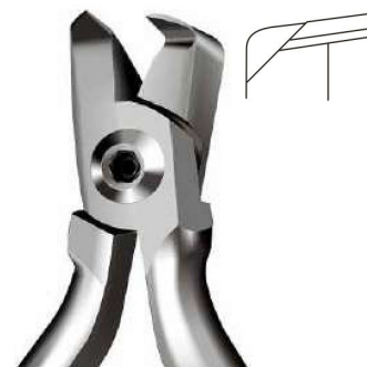
B-12-6312 T/C 11.5 cm/ 4½" Distal End Cutter with safety hold It shear cuts hard wire and braided wire and then, safely holds the loose distal ends of the wire, thus preventing from falling down into the oral tissues. The cutting edges are diamond honed. Maximum cutting capacity: rectangular and twist wires up to .022 x .028" ( 0.56 x 0.71); round wire up to .020" ( 0.51 mm) in diameter.
