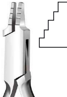
B-12-6612 Loop Closing Plier, Nance Style Box joint with 4 sectioned tip for forming various size loops in rectangular and round wires. For wires up to .028" ( 0.71 mm).
